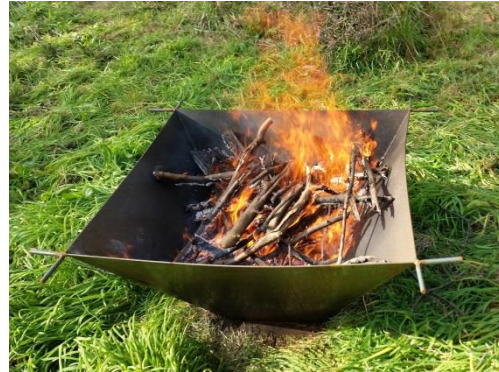
Typical flame-capped kiln for school use
