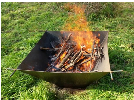
Typical flame-capped kiln for garden use
