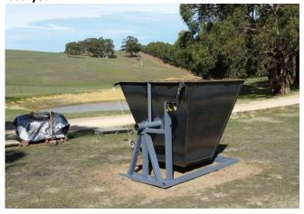
The kiln is suspended on a shaft and stand so as to clear the ground when tipped for emptying. The shaft is held in a sealed bearing housing on each side and two winches are included to enable manual tipping. The kiln has a volume of 2.12 cu.m.
