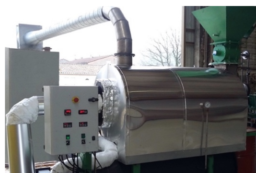
CarboChar-1 is the smallest model of the biochar production machines developed by Pro-Natura
